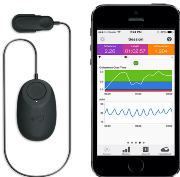
Figure 1. The Inner Balance device is a state of the art, ultra-low Bluetooth device with 125 hz sample rate measuring HRV parameters to optimise accurate HRV and QCT training.
